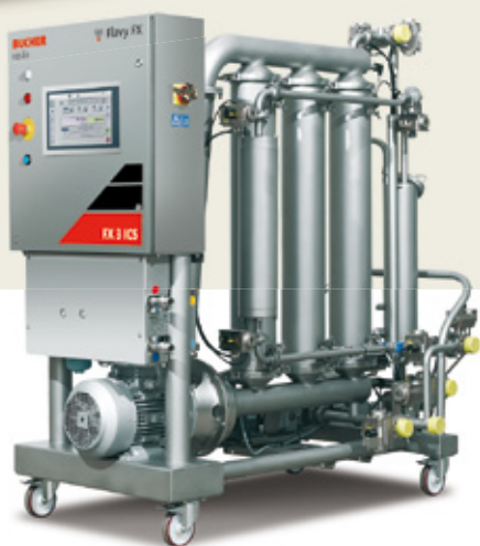
Filtre tangential Flavy FX 3 ICS
